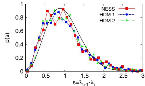
FIG. 5 (color online). LSD for two HDMs with the largest real eigenvalues  $\Lambda_1 = -0.0943$  (blue),  $\Lambda_2 = -0.1574$  (green), for the XXZ chain in a staggered field. Red points are for the NESS,  $\Lambda_0 = 0$  ( $\Delta = 0.5$ ,  $\mu = 0.1$ ,  $\bar{\mu} = 0$ ,  $\Gamma = 1$ ,  $n = 13$ ,  $Z = 7$ ). Full black curve is the Wigner surmise for the GUE.
